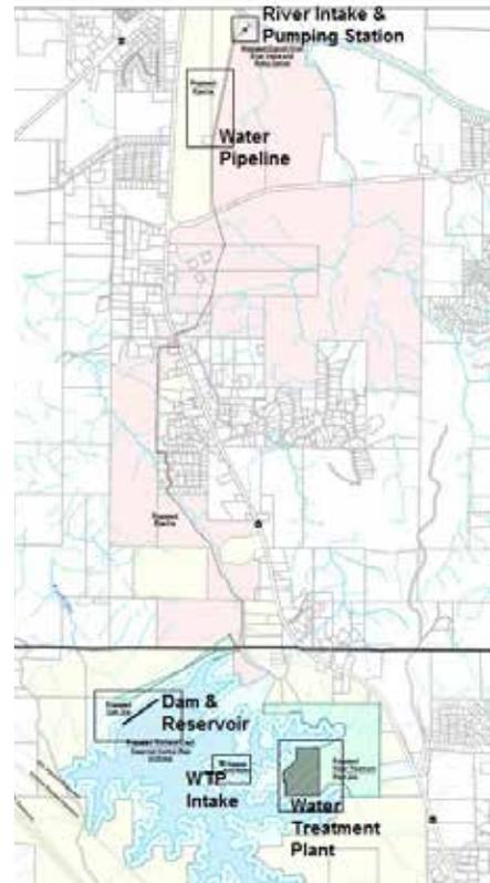
Overview of the Richland Creek Reservoir Water Supply Program. Water from the Etowah River to the north will be piped about 3.7 miles to the new reservoir. A new water treatment plant has been built and will treat water from the reservoir at an initial rate of 18 million gallons per day.
