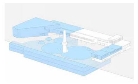
The innovative design of the new Amos Rex art museum features a subterranean gallery and an even lower level for art storage. Ever-present groundwater placed critical importance on choosing the right waterproofing solution for the foundation.
