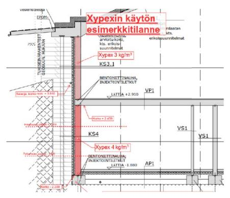
Project engineers consulted with Xypex Technical Services to determine the optimal dosing for Admix C-1000 NF waterproofing admixture based on the depth of the structure and the projected hydraulic pressure from groundwater.
